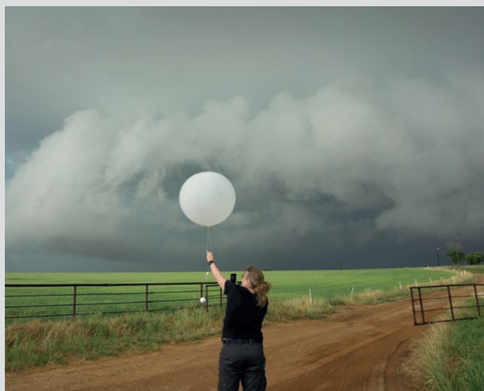
Launch of a hail probe into a supercell. (Photo: Jannick Fischer)
